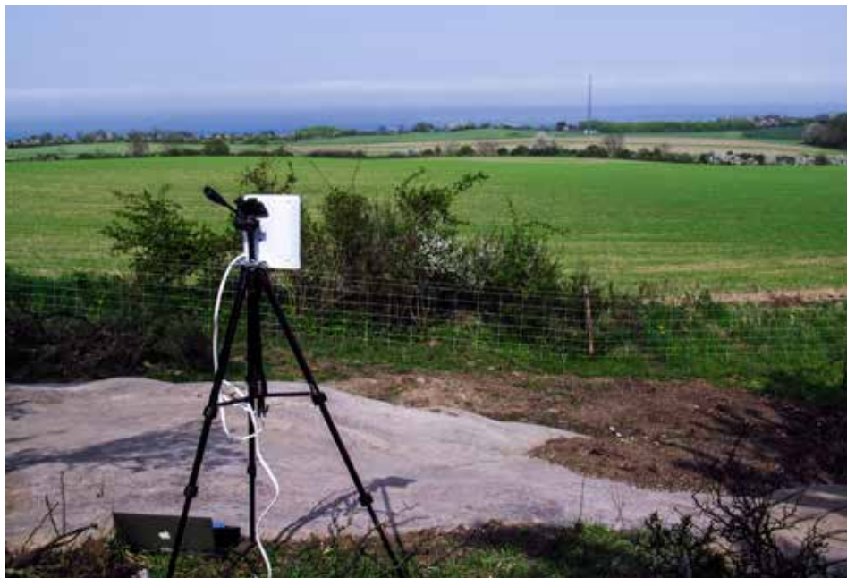
Figure 2: Field situation: laptop and wireless router connected to antenna mounted on tripod transmitting to mast in background. Upl/download speed up to 17 MB/sec for a transfer of 600 photos. BMR 2262-72 Hammersholm 72, North Bornholm (photo: author). More usual speeds in North Bornholm are between 0.7 and 3 MB/sec up and 3-7MB/sec down.
