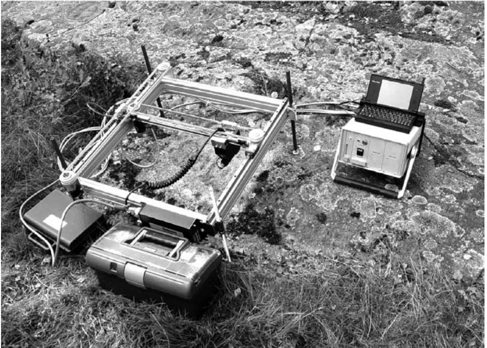
Fig. 2. The laser scanner during measurement at site 13 (Foss 6, Lökeberg) in the province of Bohuslän. There is a dense lichen growth on the veined gneiss. The two motor cycle batteries used as power source are not seen in the picture.
