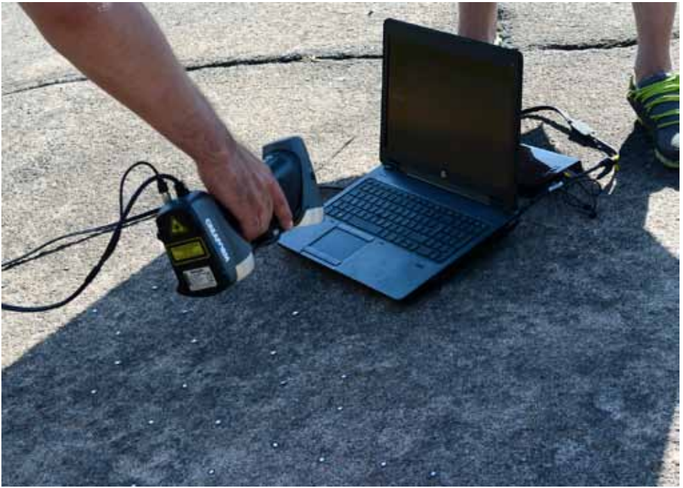
Figure 1: Documentation of a rock surface with a handheld laser scanner. Photo: Catarina Bertilsson, SHFA
